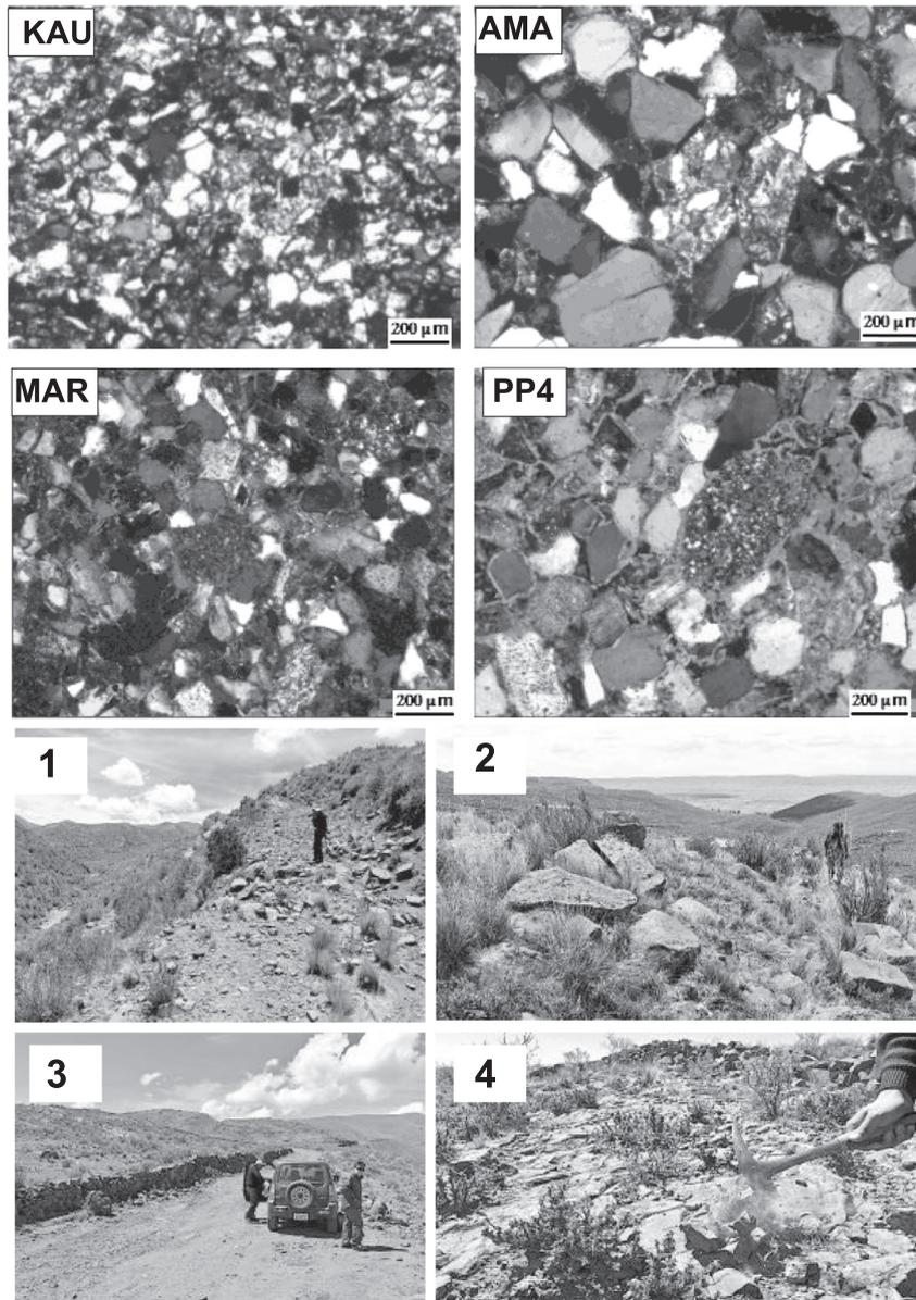
**Fig. 2.** Thin sections of sample KAU (Kausani), AMA (Amarillani), MAR (Kallamarka), PP4 (Pumapunku monument stone, fragment nr. 4). Geological sites: (1) steep llama track to KAU Kausani; (2) Kausani quadratic sandstone blocks resulting from natural weathering, geological processes of fracturing; (3) road to MAR Kallamarka; (4) MAR sampling site of easily disaggregated kaolinitized sandstone.
